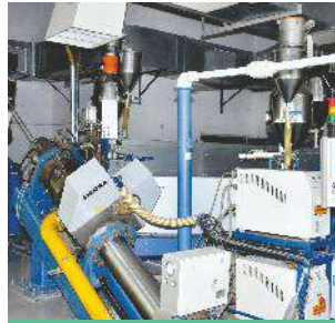
550 kV Maillefer HVCV Insulate Line
