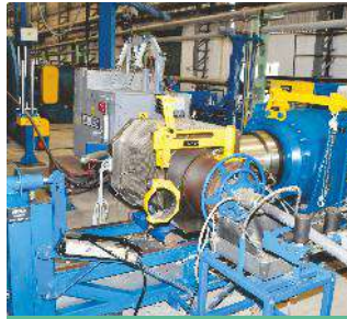
Lead Sheathing Line
