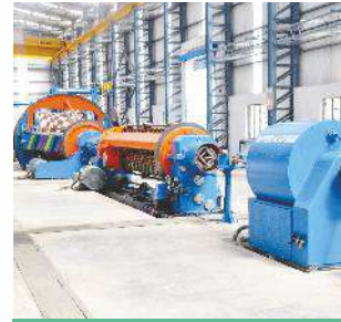
DT Armouring Machines
