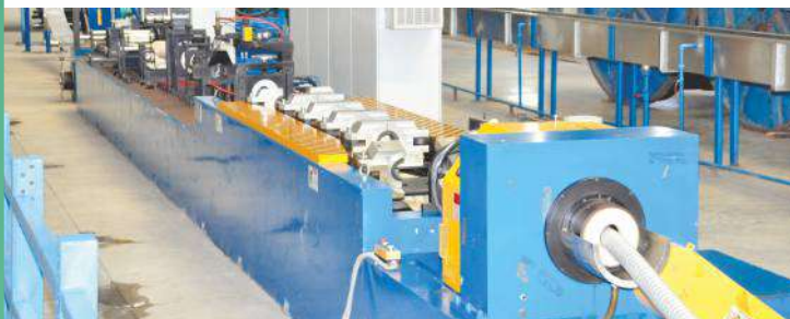
Aluminum Corrugation Line
